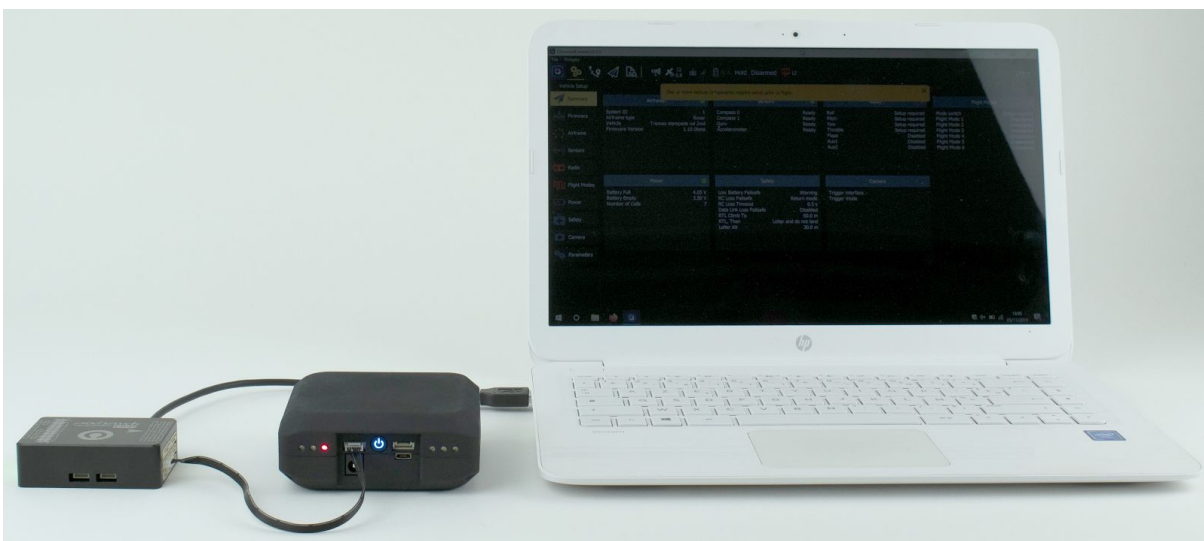
Figure 4. Sirius F9P Base connected to a Pixhawk 3 Pro autopilot and a PC running QGroundControl
